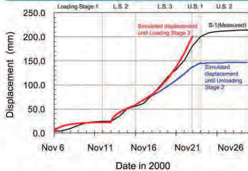
Fig. 12 Simulated and measured ground displacements. Red line, cohesion reduced from 9.1 to 5.0 kN/m 2 during loading stage 3. Blue line, cohesion reduced from 9.1 to 7.0 kN/m 2 during loading stage 3. Black line, measured displacement at S-1
