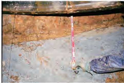
Fig. 8 Sliding surface inside the exploration shaft
